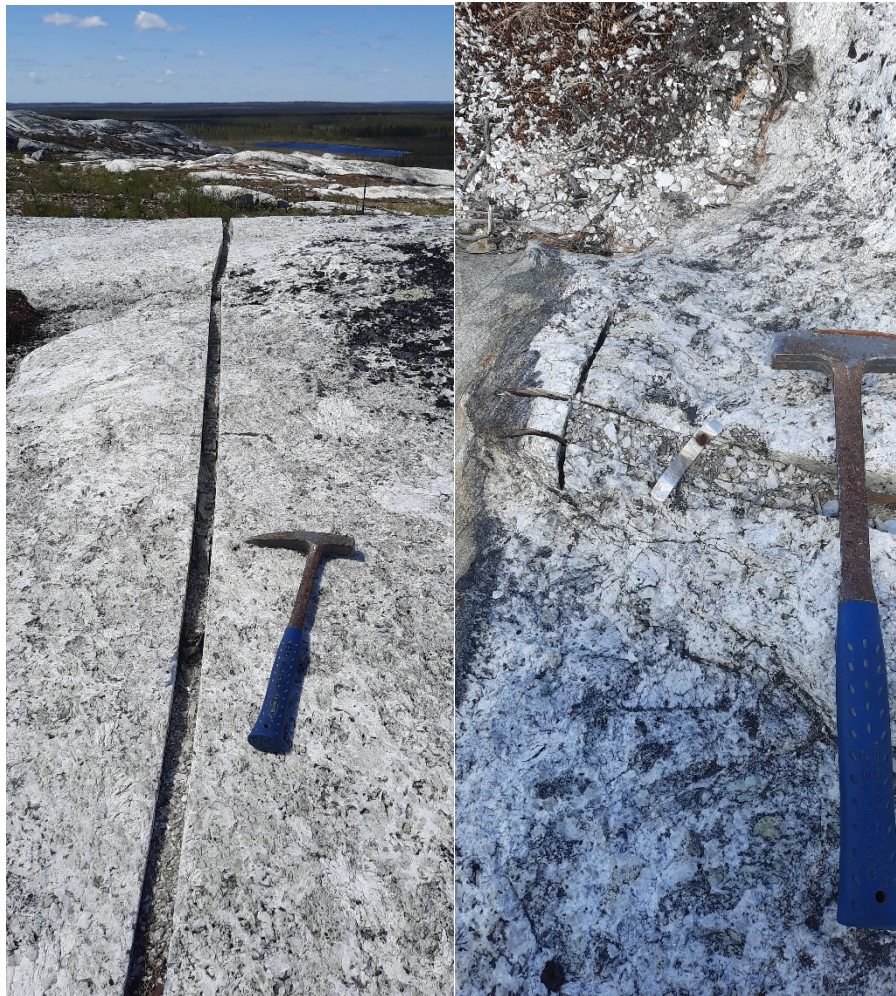
Figure 12.3: Example of Channel Sampling. Left: Channel Sample Perpendicular to Pegmatite Orientation. Right: Channel Sample Ending at Contact with Metasediments.
