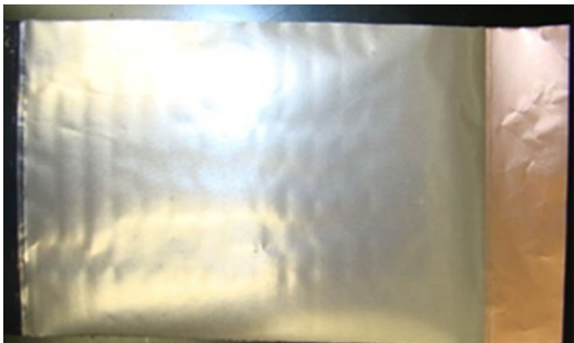
Calendered lithium metal foil sheet
